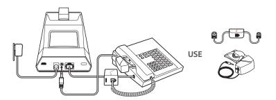
• Adjust the configuration switch on the bottom of the base to default **A**, which works for most phones. Use configuration **D** for Cisco phones.
